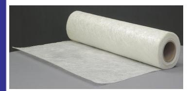
FGOC ECPlus Chopped Strand Mat 611 is manufactured by the uniform distribution of chopped ECPlus boron free-glass filament strands of  $\sim$ 50mm length, laid in a random orientation and held together by an PVAc emulsion binder. The CSM EB 611 mat offers:
