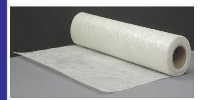
FGOC ECPlus Chopped Strand Mat 611 is manufactured by the uniform distribution of chopped ECPlus boron free-glass filament strands of  $\sim$ 50mm length, laid in a random orientation and held together by a polyester powder binder. The CSM PB 611 mat offers:
